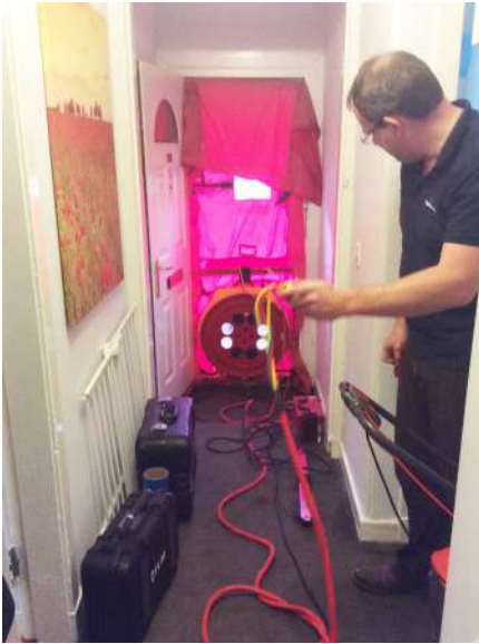
The infiltration level of a property can be established accurately using a pressurisation test, which measures how 'leaky' a building is
