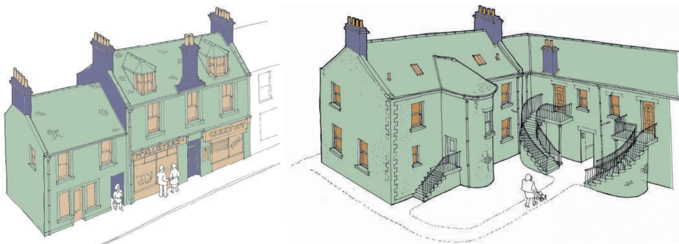
Common repairs and responsibilities: common (shown in green), individual (shown in brown) and mutual (shown in purple)
